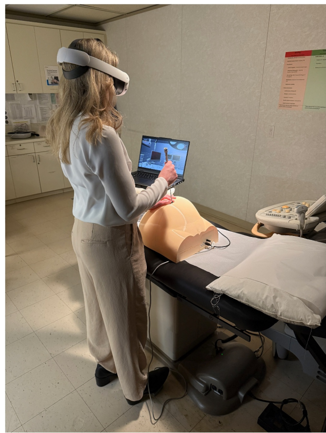
FIGURE 3 | Virtual reality simulator setup. This image demonstrates a trainee using the complete VR simulator system. The trainee wears a Meta Quest 3 Headset while manipulating the custom engineered fetoscope controller. Note the 3D-printed maternal abdomen with integrated fetoscope that provides tactile feedback for fetoscope manipulation. The foot pedal for laser activation is visible at the bottom. This integrated hardware-software system allows for a fully immersive training experience that combines physical and virtual elements to simulate the TTTS environment.
